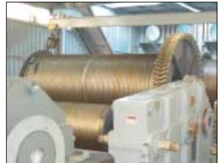
New drum and gearing made in-house by Northrop Grumman Newport News.
